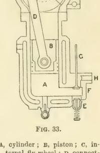
A, cylinder; B, piston; C, internal fly-wheel; D, connecting-rod; E, inlet valve for petrol vapour; F, exhaust valve; G, exhaust valve stem; H, exhaust opening.
